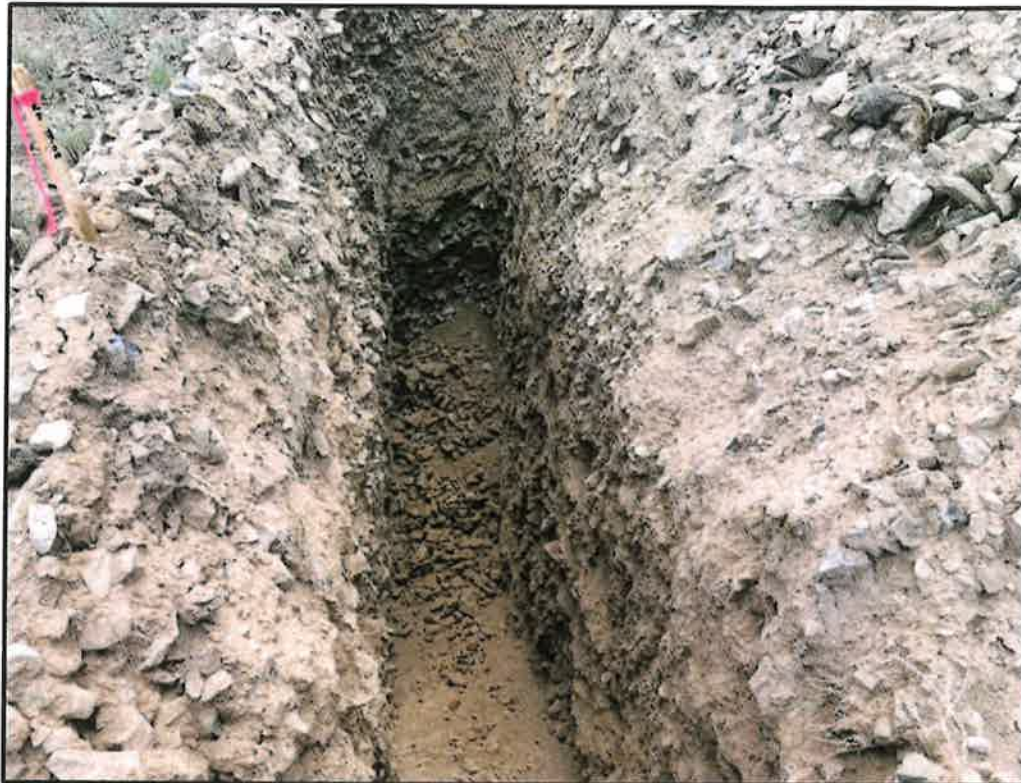
TP-08 trench profile. Note main cobble unit.
