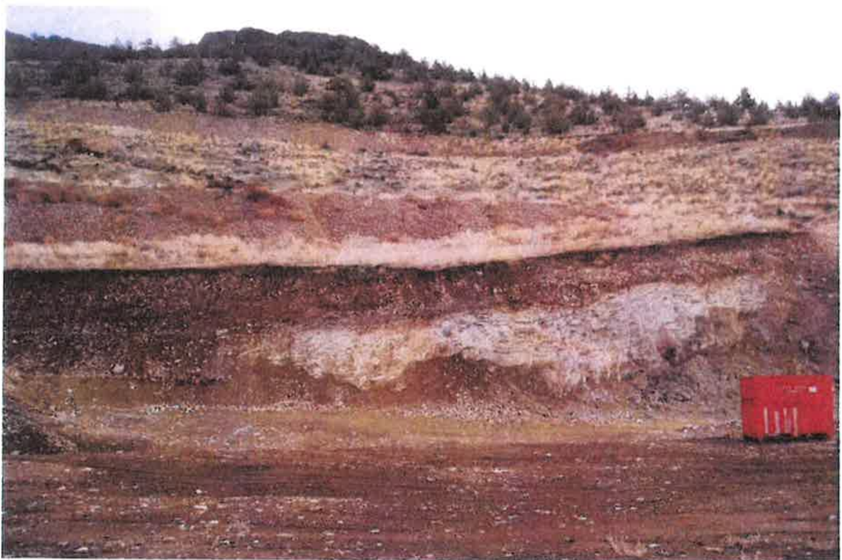
John Day Formation overlain by alluvial cobbles, lower terrace cut face, southern portion, note TP-04 spoils on hill, mid-terrace spoils and upper roadway cut spoils
